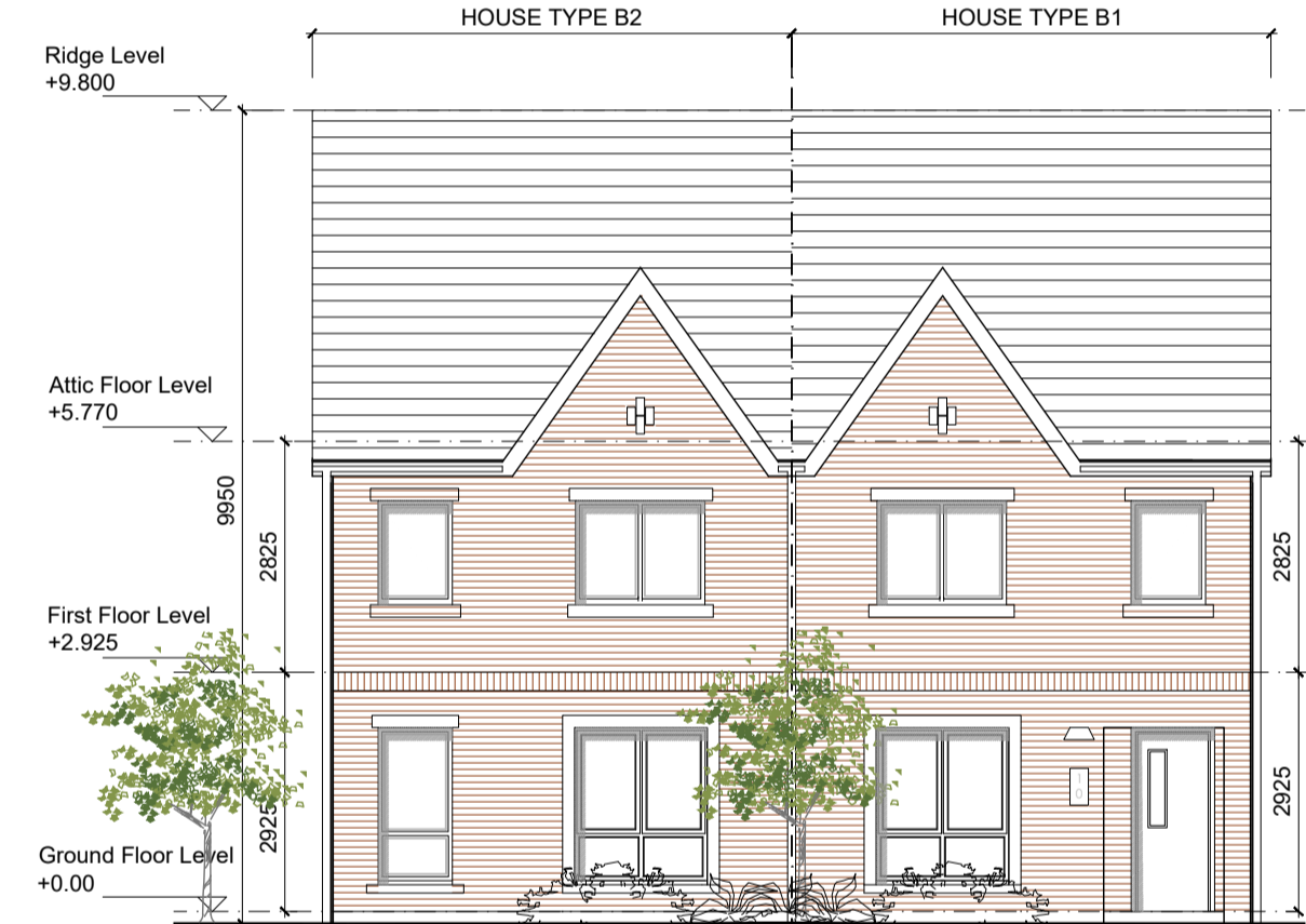
FRONT ELEVATION (Type B2-B1) Scale 1:100
