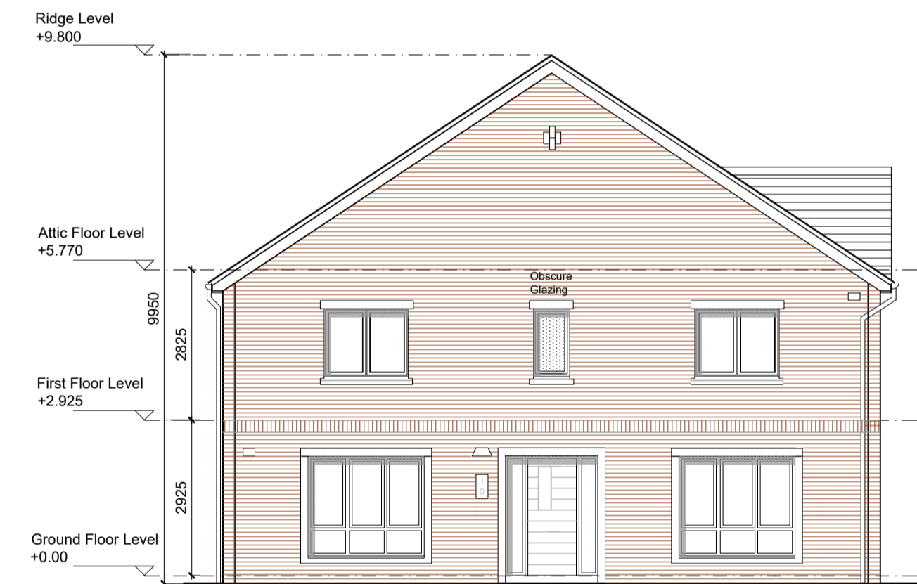
SIDE ELEVATION (Type B2) Scale 1:100 Mirrored where applicable
